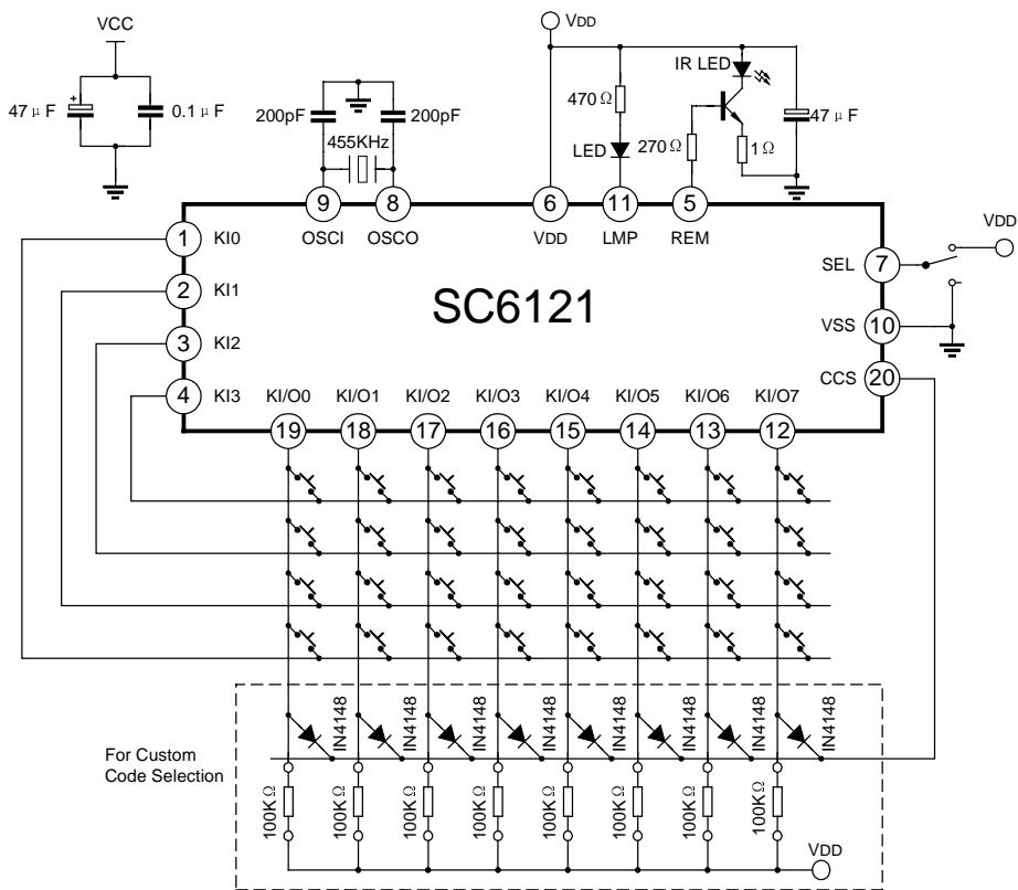
Note:1. Two capacitance connect with Vcc should as near as possible.
