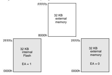
Notes: 1. If the program executes exclusively from on-chip code memory (not from external memory), beware of executing code from the upper byte of on-chip memory (7FFFh) and thereby disrupt I/O Ports 0 and 2 due to external prefetch. Fetching code constant from this location does not affect Ports 0 and 2.
