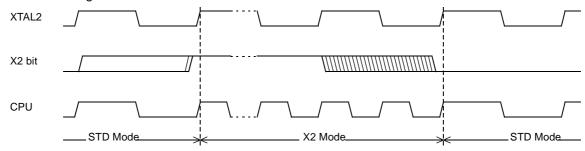
Note: In order to prevent any incorrect operation while operating in the X2 mode, users must be aware that all peripherals using the clock frequency as a time reference (UART, timers...) will have their time reference divided by two. For example a free running timer generating an interrupt every 20 ms will then generate an interrupt every 10 ms. A UART with a 4800 baud rate will have a 9600 baud rate.
