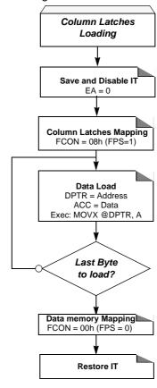
Figure 21. Column Latches Loading Procedure
