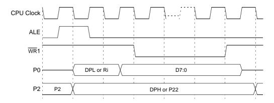
Notes: 1. WR signal may be stretched using M0 bit in AUXR register.
