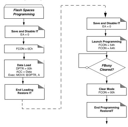
Figure 23. Hardware Programming Procedure
