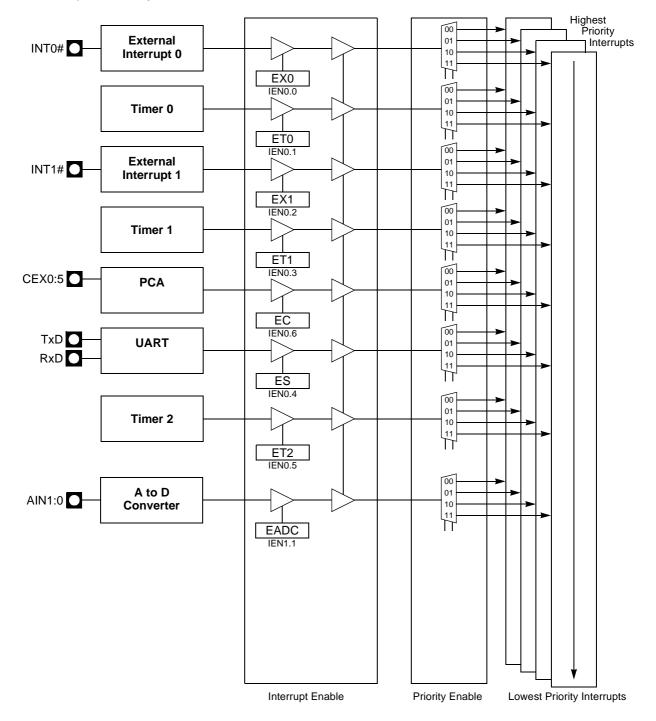
Each of the interrupt sources can be individually enabled or disabled by setting or clearing a bit in the Interrupt Enable register. This register also contains a global disable bit which must be cleared to disable all the interrupts at the same time.
