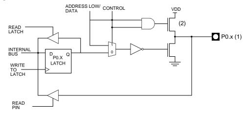
Notes: 1. Port 0 is precluded from use as general-purpose I/O Ports when used as address/data bus drivers.
