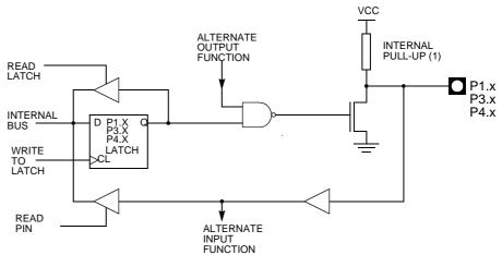
Note: The internal pull-up can be disabled on P1 when analog function is selected.
