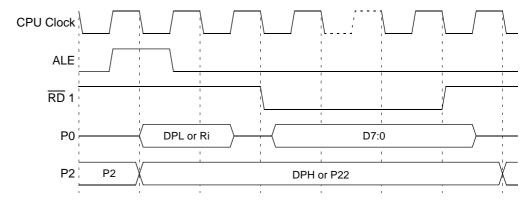
Notes: 1. RD signal may be stretched using M0 bit in AUXR register.
