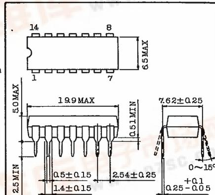
Lead pitch is 2.54 and tolerance is  $\pm 0.25$  against theoretical center of each lead that is obtained on the basis of No.1 and No.14 leads.
