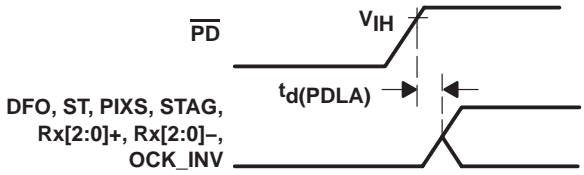
Figure 9. Delay From \overline{PD} Low to High Before Inputs Are Active
