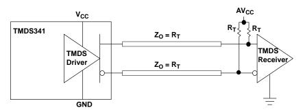
Figure 32. TMDS Driver and Termination Circuit
