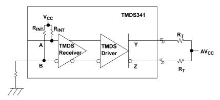
Figure 31. TMDS Input Fail-Safe Recommendation
