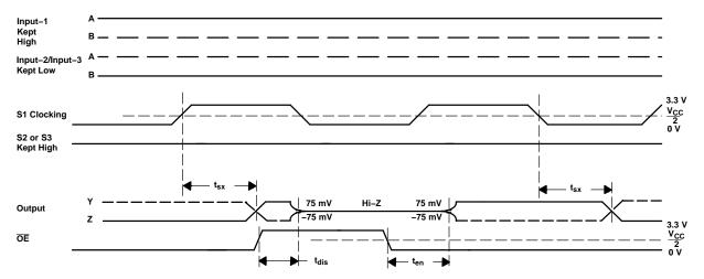
**Figure 6. TMDS Outputs Control Timing Definitions**
