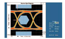
Figure 34. Eye Diagram Recovered by TMDS341 vs TP1
