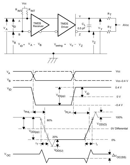
NOTE: All input pulses are supplied by a generator having the following characteristics:  $t_r$  or  $t_f$  < 100 ps, 100 MHz from Agilent 81250.  $C_L$  includes instrumentation and fixture capacitance within 0.06 m of the D.U.T. Measurement equipment provides a bandwidth of 20 GHz minimum.
