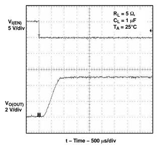
Figure 2. Turnon Delay and Rise Time With 1-µF Load
