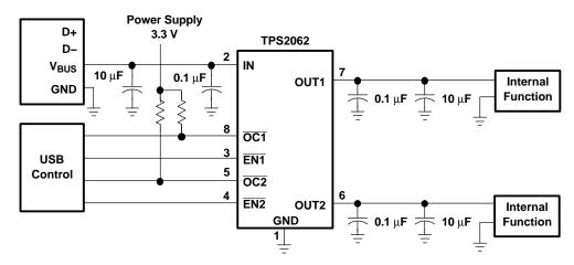
Figure 28. High-Power Bus-Powered Function
