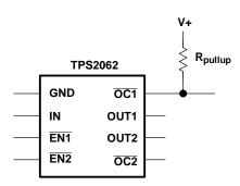
Figure 26. Typical Circuit for the OC Pin
