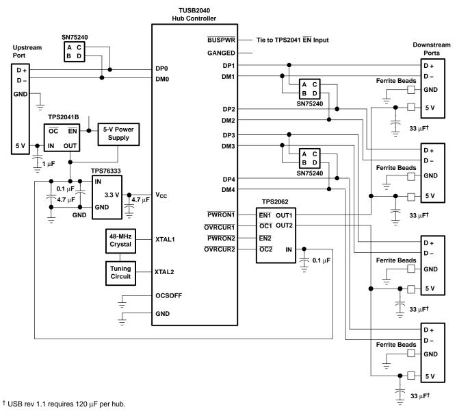
Figure 29. Hybrid Self / Bus-Powered Hub Implementation
