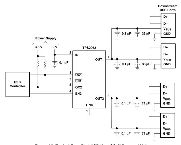
Figure 27. Typical Four-Port USB Host / Self-Powered Hub
