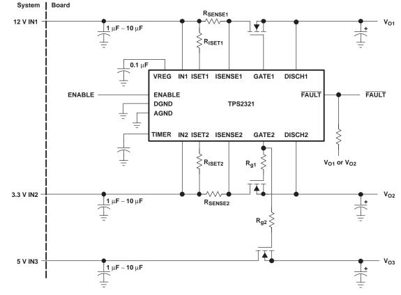
Figure 27. Three-Channel Application
