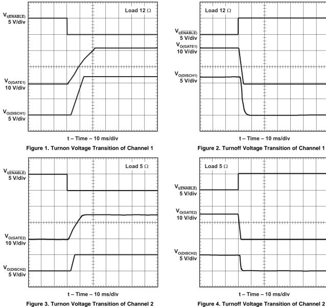
Figure 3. Turnon Voltage Transition of Channel 2
