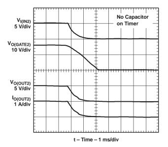
Figure 14. Channel 2 - Hot Removal
