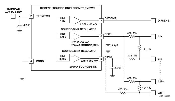
Figure 1. Low-Voltage Differential Discrete Resistor Stack
