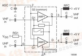
V<sub>GG</sub> = 5 V: UHF AMP is on; VHF AMP is off V<sub>GG</sub> = 0 V: UHF AMP is off; VHF AMP is on (0 = shorted to Ground or open)
