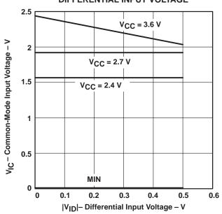
Figure 1.  $V_{IC}$  vs  $V_{ID}$  and  $V_{CC}$
