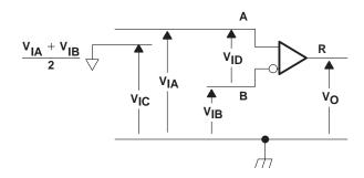
Figure 2. Receiver Voltage Definitions
