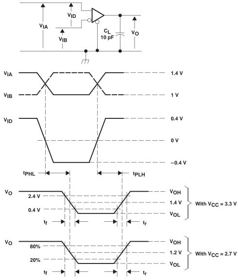
NOTE A: All input pulses are supplied by a generator having the following characteristics:  $t_f$  or  $t_f \le 1$  ns, pulse repetition rate (PRR) = 50 Mpps, pulse width =  $10 \pm 0.2$  ns.  $C_L$  includes instrumentation and fixture capacitance within 0,06 m of the D.U.T.
