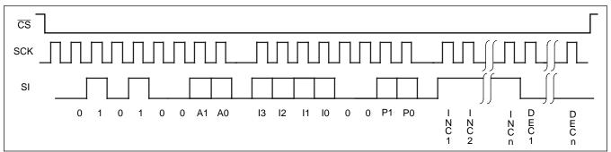
Figure 8. Increment/Decrement Timing Limits
