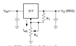
$V_O (REG) = 1.25V (1+R_2/R_1)+I_{adj} R_2$
