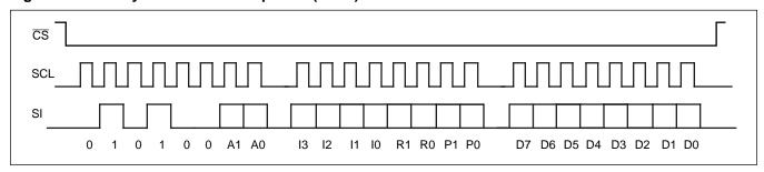
Figure 6. Three-Byte Instruction Sequence (Read)
