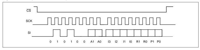
Figure 5. Three-Byte Instruction Sequence (Write)
