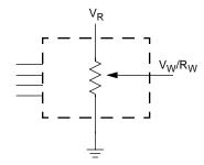
Three terminal Potentiometer; Variable voltage divider
