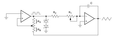
$\begin{array}{l} frequency \propto R_1, \, R_2, \, C \\ amplitude \propto R_A, \, R_B \end{array}$
