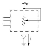
Two terminal Variable Resistor; Variable current
