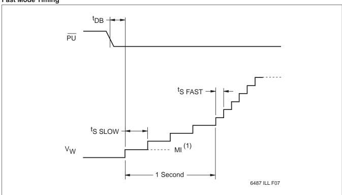
$\textbf{Notes:} \hspace{0.1in} \textbf{(1) MI in the A.C. timing diagram refers to the minimum incremental change in the wiper voltage.} \\$
