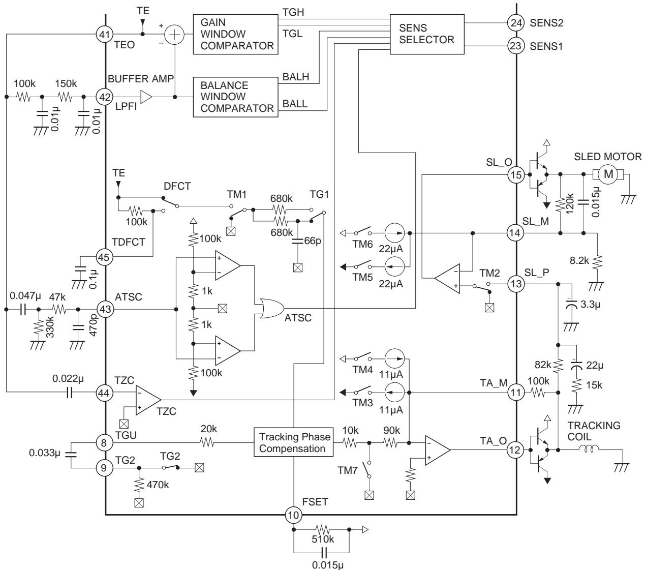
The above figure shows a block diagram of the tracking and sled servo.
