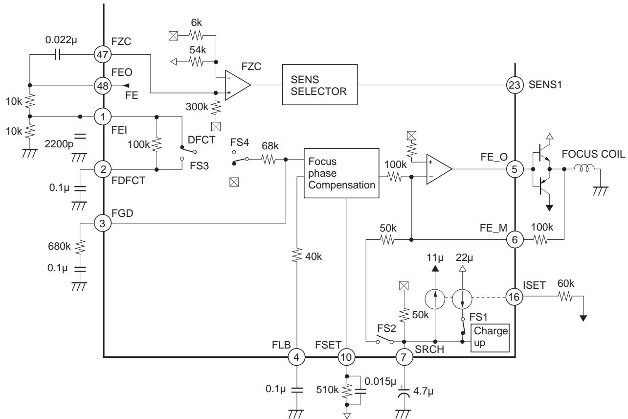
The above figure shows a block diagram of the focus servo.
