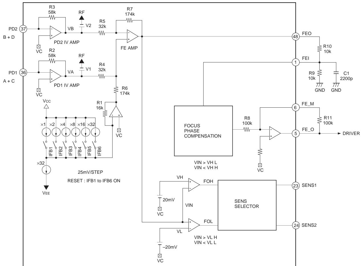
The focus error amplifier calculates the difference between outputs VA and VB of the RF I-V amplifier, and outputs current-voltage converted voltage of the photodiode (A + C – B – D).
