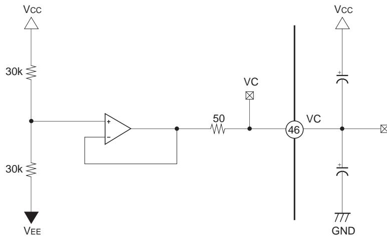
Connected internally to the VEE pin.
