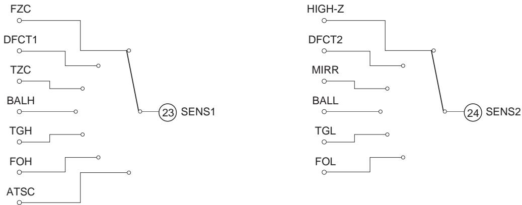
What is output to the SENS1 and SENS2 pins varies according to the address input to the DATA pin.
