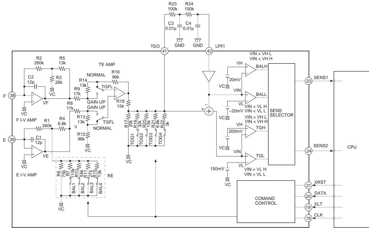
The difference between E I-V amplifier output VE and F I-V amplifier output VF is taken and output from TEO.
