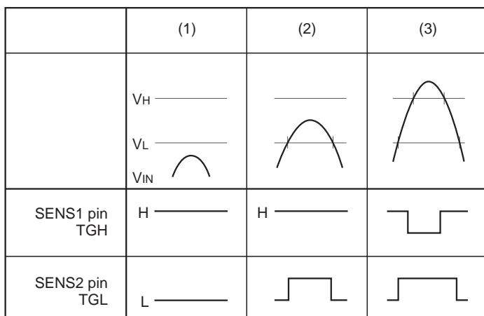
The gain should be adjusted so that the SENS1 and SENS2 pins are as shown in status (2).
