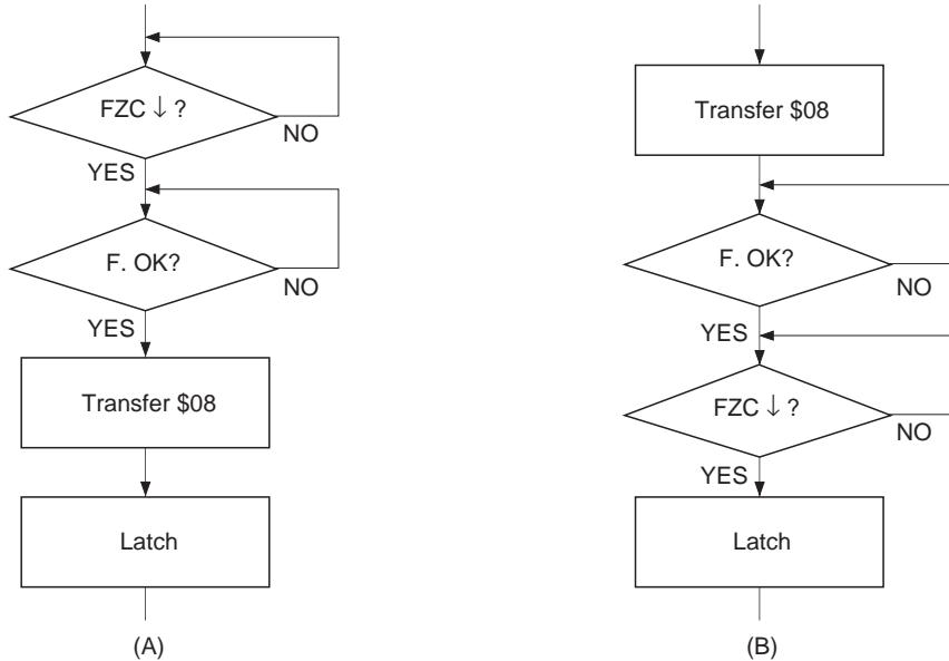
**Fig. 5. Poor and good software command sequences**
