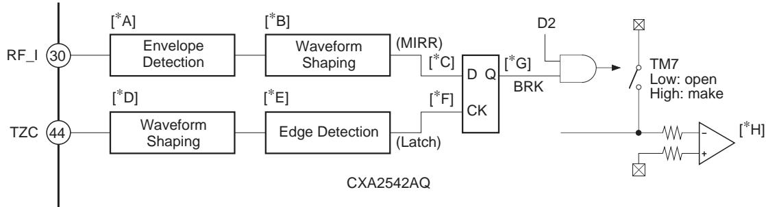
**Fig. 6. TM7 movement during braking operation**
