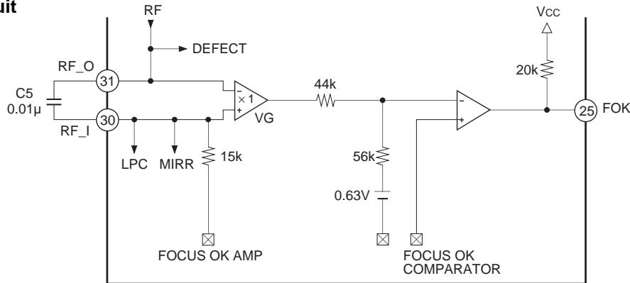
The focus OK circuit creates the timing window okaying the focus servo from the focus search state.
