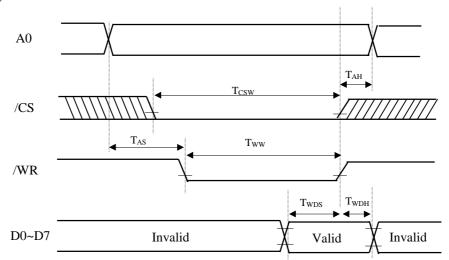
Note:  $T_{CSW}$ ,  $T_{WW}$ ,  $T_{WDH}$  and  $T_{AH}$  are defined with respect to the moment /CS or /WR becomes High level.
