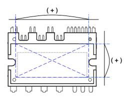
Figure 5. Flatness Measurement Position
