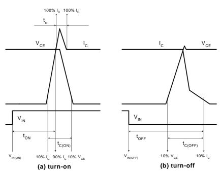
Figure 4. Switching Time Definition
