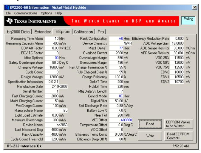
To read all the data from the bq2060A EEPROM click on | Read |. To write to a selected location, click on the desired location, type in the desired data, and press the ENTER key. After a moment, the next location is highlighted. The entire EEPROM can be written this way.
