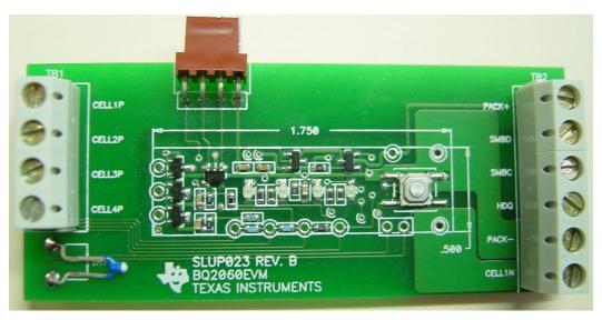
This EVM is a complete evaluation system for the bq2060A battery management system. The bq2060A is backwards compatible with the bq2060. New features in the bq2060A can be accessed from the EEPROM screen in the EV2200-60 software.
