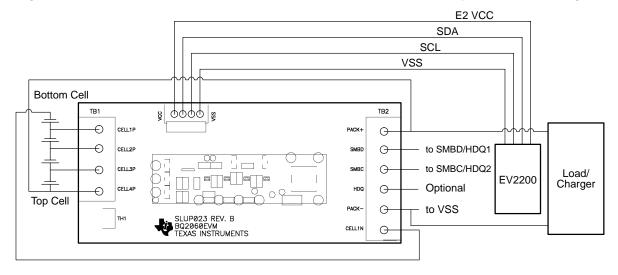
Figure 4–2. bq2060A Circuit Module Connection to NiMH Cells and System Load/Charger
