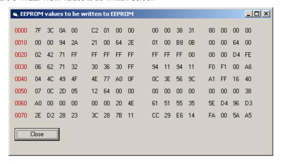
All data required for calibration is also held in the EEPROM for the bq2060A as highlighted in Figure 5–8.
