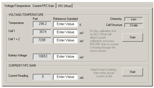
The LiON Calibration screen differs from the NiMH calibration screen by the individual cell voltages and cell structure. If the Chemistry or Cell Structure fields do not show the proper configuration in their respective fields, then select the bq2060A Data Screen Tab, select | Options | Initialize Device |, wait 5 seconds and then return to the Calibration Tab.
