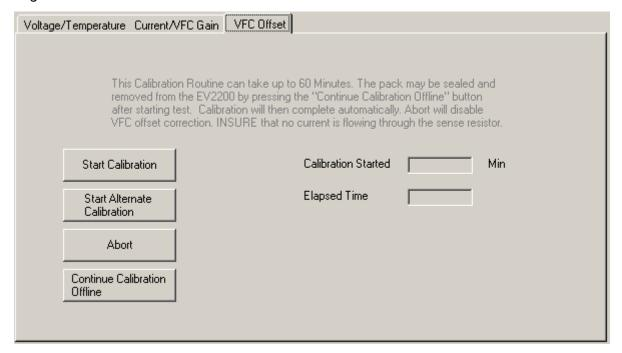
Default VFC Offset: To select this offset method, click on | Start Calibration |. This method appies an internal short (inside the bq2060A) across the sense resistor. With the sense resistor shorted inside the bq2060A, there is less chance that an external current can cause a poor offset calculation. If the circuit board induces a slight offset, then it is not compensated for with this method.
