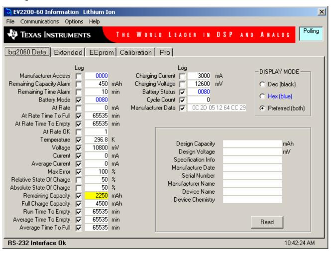
This screen shows the SBS data set along with additional Static data which is shown in a box in the bottom right quadrant. By clicking on the *Read* button, the box changes to show the static data from the bq2060A (see Figure 5–2).
