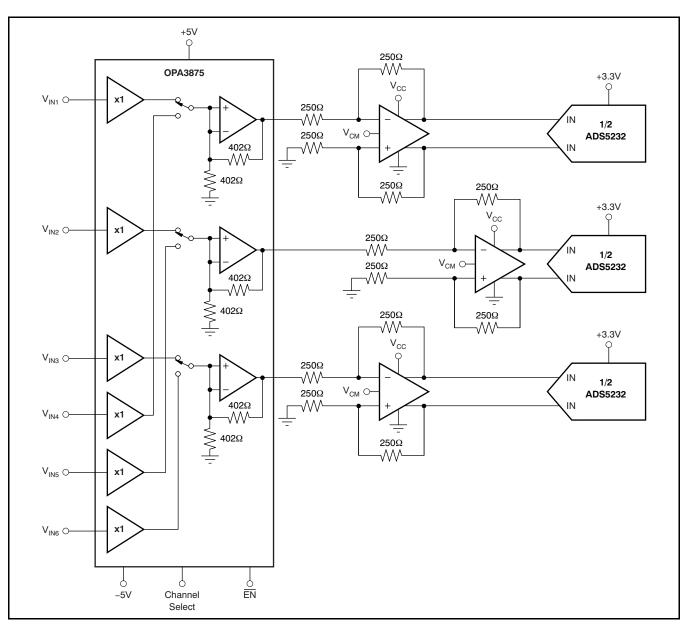
Figure 29. ADC Input Multiplexer
