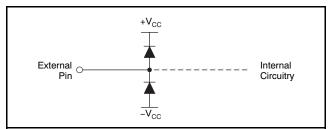
**Figure 31. Internal ESD Protection**
