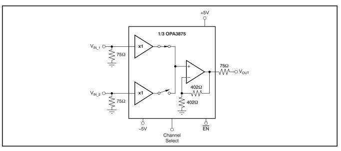
Figure 26. Triple 2:1 High-Speed Video Multiplexer
