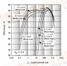
Figure 2. Efficiency vs Load Current
