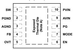
A. The exposed Thermal Die is connected to AGND.
