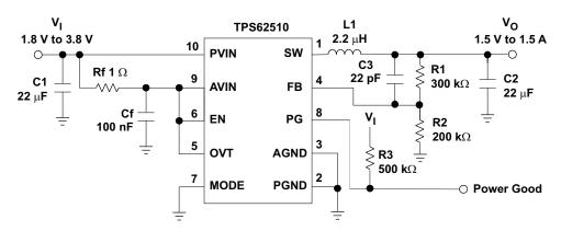
Figure 24. Adjustable Version Programmed to 1.5 V Using Power Good Revision History
