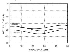
[1] Data taken with die mounted to plate and RF probed through two 1 mil diameter wire bonds.
