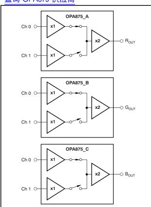
Figure 27. High Isolation RGB Video MUX
