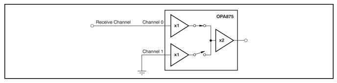
Figure 26. Transmit/Receive Switch
