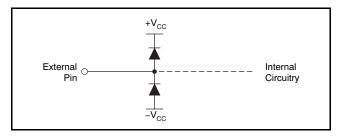
Figure 31. Internal ESD Protection
