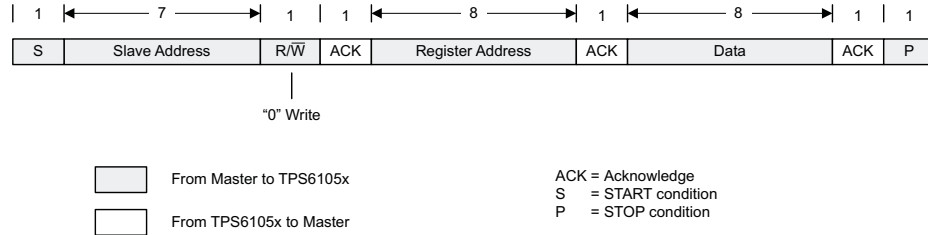
Figure 46. Write Data Transfer Format in F/S-Mode
