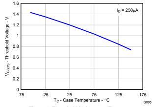
Figure 6. Threshold Voltage vs. Temperature
