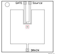
Max  $R_{\theta JA} = 57^{\circ} C/W$  when mounted on 1 inch² (6.45 cm²) of 2-oz. (0.071-mm thick) Cu.
