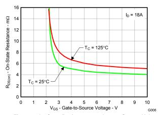
Figure 7. On-State Resistance vs. Gate-to-Source Voltage
