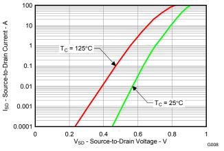
Figure 9. Typical Diode Forward Voltage
