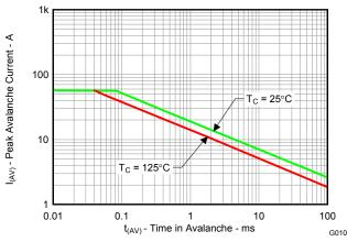
Figure 11. Single Pulse Unclamped Inductive Switching
