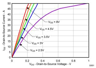
Figure 2. Saturation Characteristics
