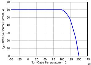
Figure 12. Maximum Drain Current vs. Temperature
