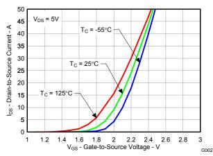
Figure 3. Transfer Characteristics
