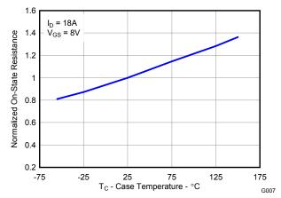
Figure 8. Normalized On-State Resistance vs. Temperature
