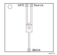
Max  $R_{\theta JA} = 174^{\circ} C/W$  when mounted on a minimum pad area of 2-oz. (0.071-mm thick) Cu.
