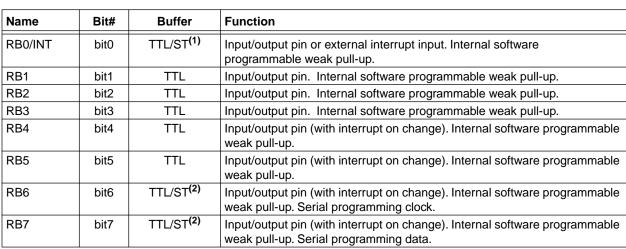
Legend: TTL = TTL input, ST = Schmitt Trigger input
