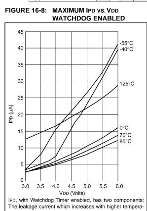
The leakage current which increases with higher temperature and the operating current of the Watchdog Timer logic which increases with lower temperature. At -40°C, the latter dominates explaining the apparently anomalous behavior.
