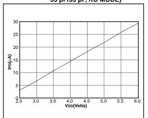
FIGURE 12-11: MAXIMUM IPD vs. TIMER1 ENABLED (32 kHz, RC0/RC1 = 33 pF/33
