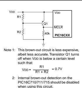
3: Resistors should be adjusted for the characteristics of the transistor.
