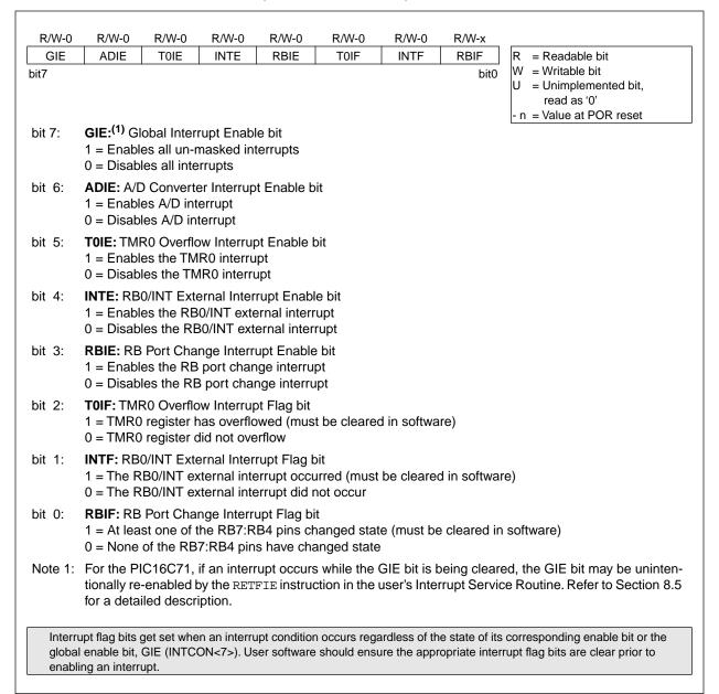
**Note:** Interrupt flag bits get set when an interrupt condition occurs regardless of the state of its corresponding enable bit or the global enable bit, GIE (INTCON<7>).
