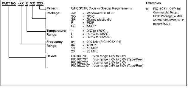
\* JW Devices are UV erasable and can be programmed to any device configuration. JW Devices meet the electrical requirement of each oscillator type (including LC devices).
