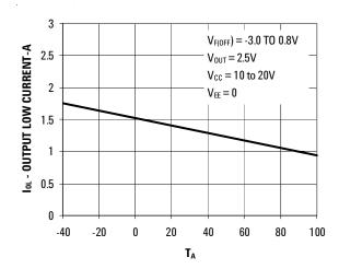
Figure 5.  $I_{OL}$  Vs Temperature
