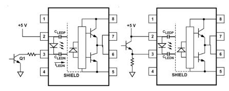
Figure 32. Not Recommended Open Collector Drive Circuit.
