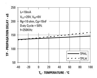
Figure 12. Propagation Delay Vs Temperature
