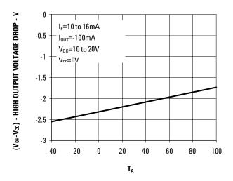
Figure 1. V<sub>OH</sub> Vs Temperature
