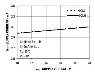
Figure 8. I $_{CC}$  Vs V $_{CC}$
