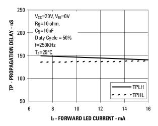
Figure 11. Propagation Delay Vs IF
