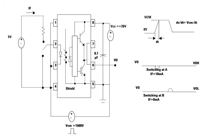
Figure 24. CMR Test Circuit and Waveform
