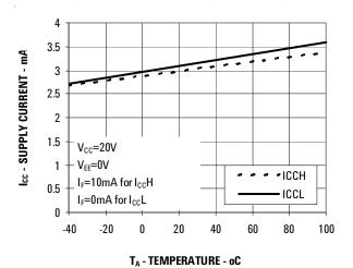
Figure 7. I<sub>CC</sub> Vs Temperature
