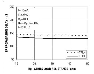
Figure 13. Propagation Delay Vs Rg
