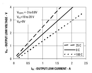
Figure 6.  $V_{0L} Vs I_{0L}$
