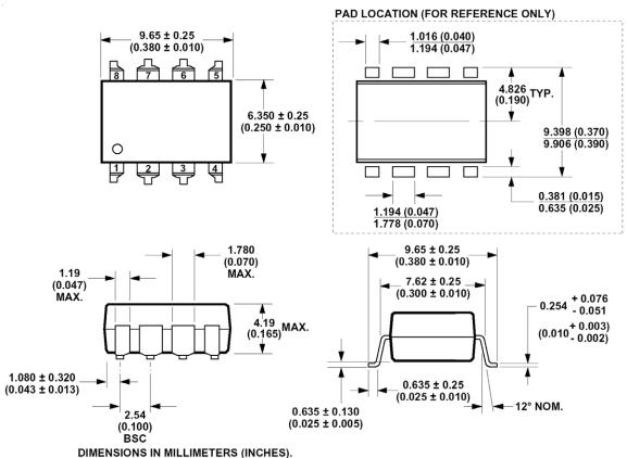
DIMENSIONS IN MILLIMETERS (INCHES). LEAD COPLANARITY = 0.10 mm (0.004 INCHES).
