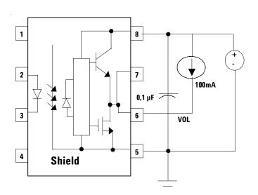
Figure 20. VOL Test Circuit
