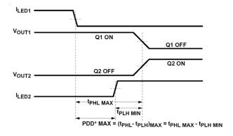
\*PDD = PROPAGATION DELAY DIFFERENCE NOTE: FOR PDD CALCULATIONS THE PROPAGATION DELAYS ARE TAKEN AT THE SAME TEMPERATURE AND TEST CONDITIONS.
