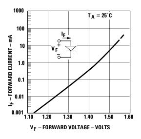
Figure 16. Input Current Vs Forward Voltage
