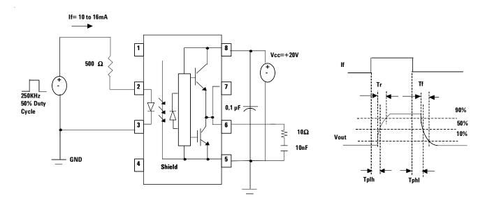
Figure 23. TPLH, TPHL, Tr and Tf Test Circuit and Waveform
