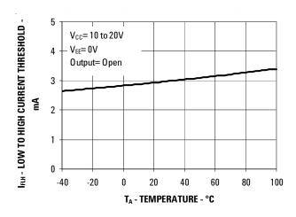
Figure 9. IFLH Vs Temperature
