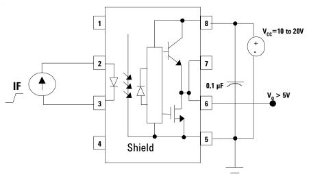
Figure 21. IFLH Test Circuit
