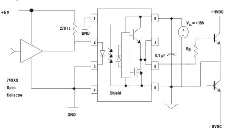
Figure 25. Recommended LED Drive and Application Circuit for HCPL-3180
