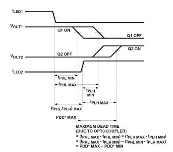
\*PDD = PROPAGATION DELAY DIFFERENCE NOTE: FOR DEAD TIME AND PDD CALCULATIONS ALL PROPAGATION DELAYS ARE TAKEN AT THE SAME TEMPERATURE AND TEST CONDITIONS.
