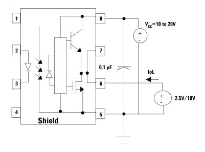
Figure 18. IOL Test Circuit
