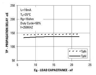
Figure 14. Propagation Delay Vs Cg
