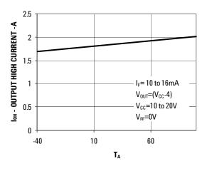
Figure 2. I<sub>OH</sub> Vs Temperature
