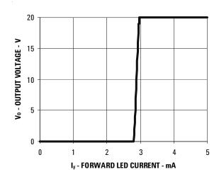
Figure 15. Transfer Characteristics
