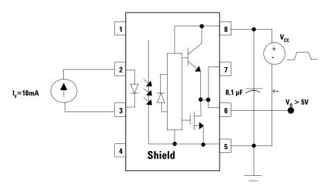
Figure 22. UVLO Test Circuit
