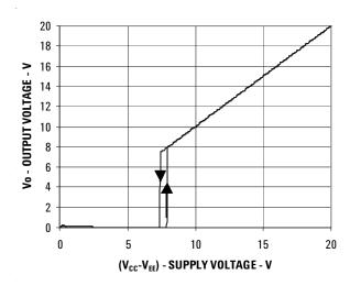
Figure 34. Under Voltage Lock Out
