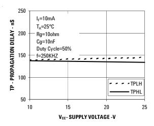
Figure 10. Propagation Delay Vs  $V_{CC}$
