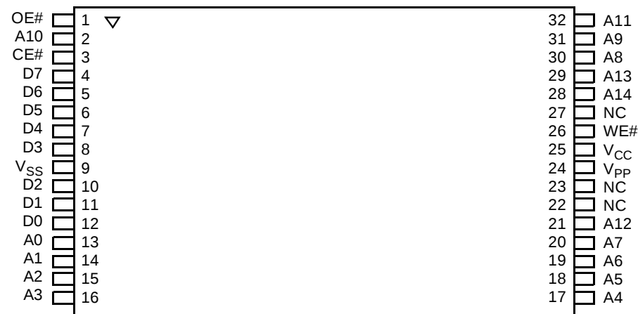
32-Pin TSOP—Reverse Pinout
