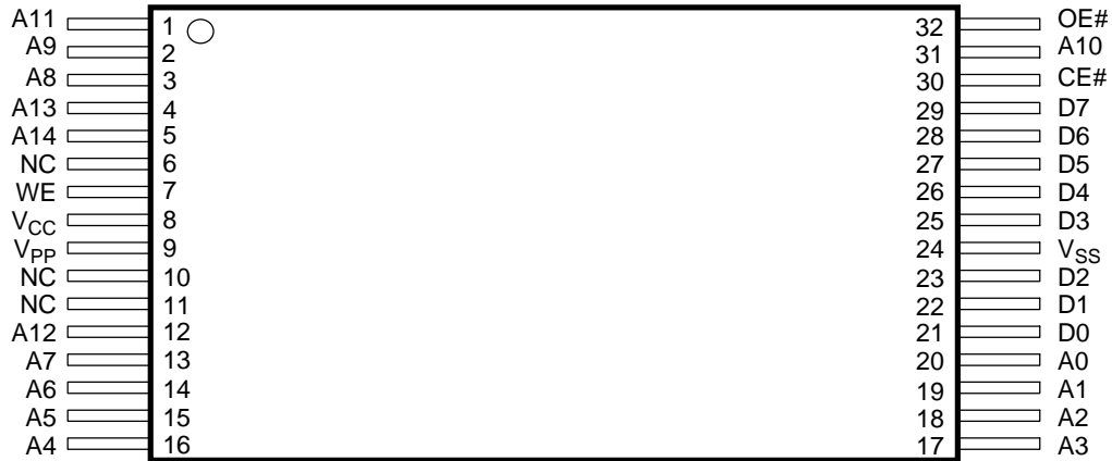
32-Pin — Standard Pinout
