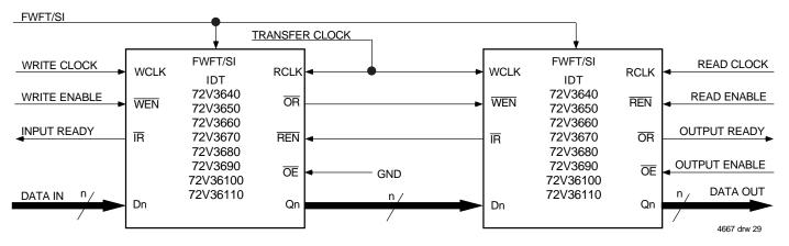
Figure 24. Block Diagram of 2,048 x 36, 4,096 x 36, 8, 192 x 36, 16,384 x 36, 32,768 x 36, 65,536 x 36, 131,072 x 36 and 262,144 x 36 Depth Expansion
