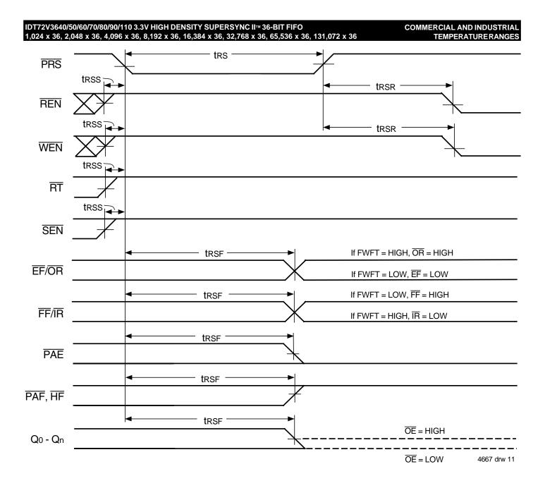
Figure 6. Partial Reset Timing
