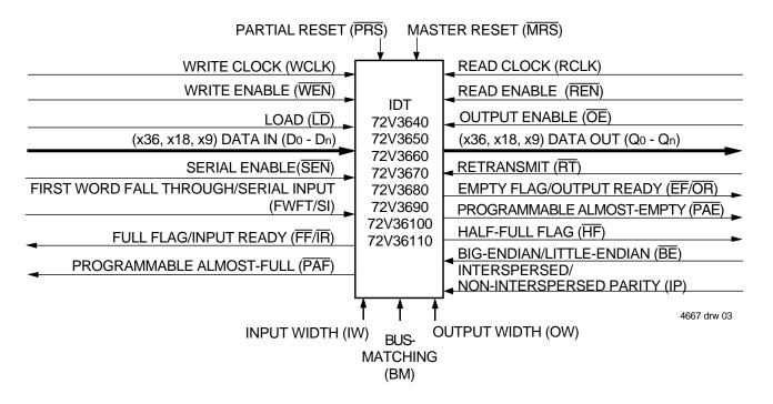
Figure 1. Single Device Configuration Signal Flow Diagram
