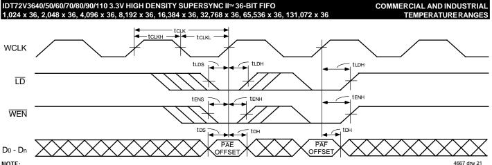
1. This timing diagram illustrates programming with an input bus width of 36 bits.
