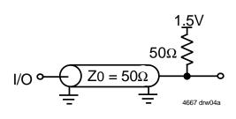
Figure 2b. AC Test Load
