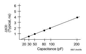
Figure 2c. Lumped Capacitive Load, Typical Derating
