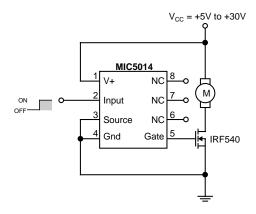
Figure 6: DC Motor Speed Control/Driver
