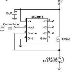
Figure 8. Halogen Lamp Driver
