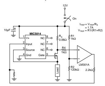
Figure 4. High Side Driver with Overcurrent Shutdown
