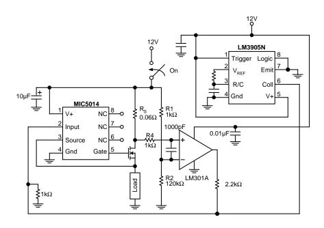
Figure 5. High Side Driver with Delayed Overcurrent Shutdown
