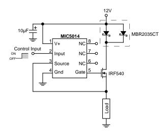
Figure 12: High Side Driver WIth Load Protection
