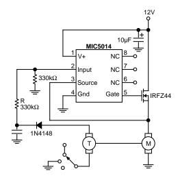
Figure 10. Motor Stall Shutdowm
