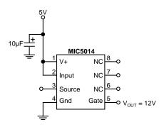
Figure 11. DC - DC Converter
