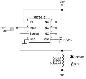
Figure 7: Solenoid Valve Driver
