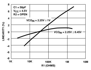
FIGURE 34. HC4046A VCO LINEARITY vs R1 (V<sub>CC</sub> = 4.5V)
