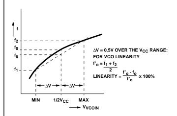
FIGURE 33. DEFINITION OF VCO FREQUENCY LINEARITY
