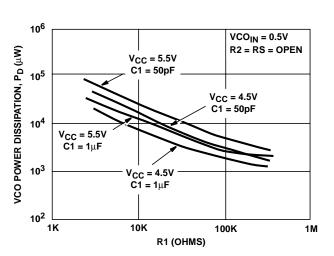
FIGURE 41. HCT4046A VCO POWER DISSIPATION vs R2 (C1 = 50pF,  $1\mu$ F)
