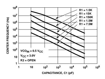
FIGURE 13. HC4046A TYPICAL CENTER FREQUENCY vs R1, C1 (V<sub>CC</sub> = 3V, R2 = OPEN)
