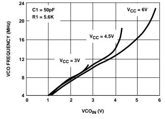
FIGURE 21. HC4046A TYPICAL VCO FREQUENCY vs VCO<sub>IN</sub> (R1 =  $5.6k\Omega$ , C1 = 50pF)
