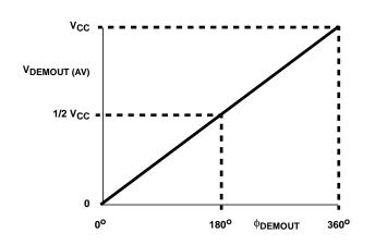
FIGURE 6. PHASE COMPARATOR 3: AVERAGE OUTPUT VOLTAGE vs INPUT PHASE DIFFERENCE: VDEMOUT = VPC3OUT
