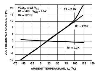
FIGURE 26. HC4046A TYPICAL CHANGE IN VCO FREQUENCY VS AMBIENT TEMPERATURE AS A FUNCTION OF R1 (V<sub>CC</sub> = 4.5V)
