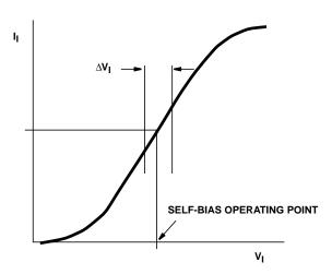
FIGURE 10. TYPICAL INPUT RESISTANCE CURVE AT  $SIG_{IN}$ ,  $COMP_{IN}$
