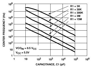
FIGURE 15. HCT4046A TYPICAL CENTER FREQUENCY vs R1, C1 (V<sub>CC</sub> = 5.5V)
