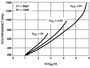
FIGURE 20. HC4046A TYPICAL VCO FREQUENCY vs VCO<sub>IN</sub> (R1 = 150k $\Omega$ , C1 = 50pF)
