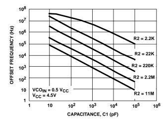
FIGURE 29. HCT4046A OFFSET FREQUENCY vs R2, C1 (V<sub>CC</sub> = 4.5V)
