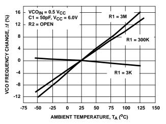
FIGURE 24. HC4046A TYPICAL CHANGE IN VCO FREQUENCY VS AMBIENT TEMPERATURE AS A FUNCTION OF R1 (V<sub>CC</sub> = 6V)
