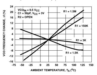
FIGURE 22. HC4046A TYPICAL CHANGE IN VCO FREQUENCY VS AMBIENT TEMPERATURE AS A FUNCTION OF R1 ( $V_{CC}$  = 3V)
