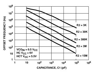
FIGURE 30. HC4046A AND HCT4046A OFFSET FREQUENCY vs R2, C1 ( $V_{CC}$  = 6V,  $V_{CC}$  = 5.5V)
