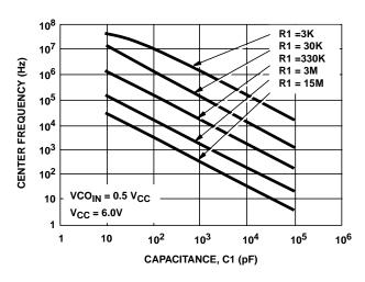
FIGURE 12. HC4046A TYPICAL CENTER FREQUENCY vs R1, C1 (V<sub>CC</sub> = 6V)
