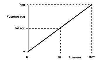
FIGURE 2. PHASE COMPARATOR 1: AVERAGE OUTPUT VOLTAGE vs INPUT PHASE DIFFERENCE:  $V_{DEMOUT} = V_{PC1OUT} = (V_{CC}/\pi) \; (\phi SIG_{IN} - \phi COMP_{IN}); \; \phi_{DEMOUT} = (\phi SIG_{IN} - \phi COMP_{IN})$
