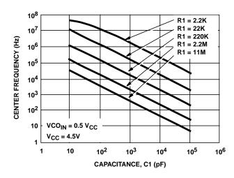
FIGURE 11. HC4046A TYPICAL CENTER FREQUENCY vs R1, C1 (V<sub>CC</sub> = 4.5V)
