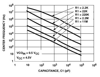
FIGURE 14. HCT4046A TYPICAL CENTER FREQUENCY vs R1, C1 (V<sub>CC</sub> = 4.5V)
