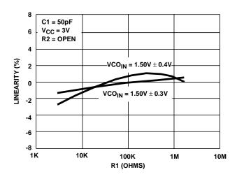
FIGURE 35. HC4046A VCO LINEARITY vs R1 (V<sub>CC</sub> = 3V)
