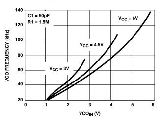
FIGURE 16. HC4046A TYPICAL VCO FREQUENCY vs VCO<sub>IN</sub> (R1 = 1.5M $\Omega$ , C1 = 50pF)
