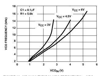
FIGURE 19. HC4046A TYPICAL VCO FREQUENCY vs VCO<sub>IN</sub> (R1 =  $5.6k\Omega$ , C1 =  $0.1\mu$ F)
