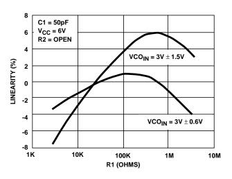
FIGURE 36. HC4046A VCO LINEARITY vs R1 (V<sub>CC</sub> = 6V)
