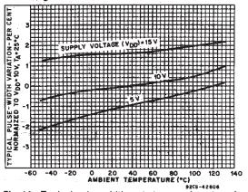
Fig. 11 - Typical pulse-width variation as a function of temperature (R<sub>x</sub>=100 KΩ, C<sub>x</sub>=2000 pF).
