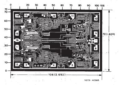
Dimensions in parentheses are in millimeters and are derived from the basic inch dimensions as indicated. Grid graduations are in mils  $(10^{-3} \text{ inch})$ .
