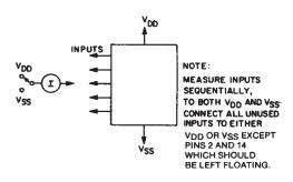
Fig. 15 - Input leakage-current test circuit.
