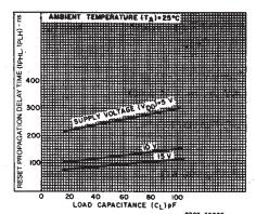
Fig. 7 - Typical propagation delay time as a function of load capacitance (RESET to Q or Q).
