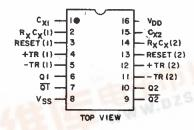
TERMINALS 1,8,15 ARE ELECTRICALLY CONNECTED INTERNALLY
