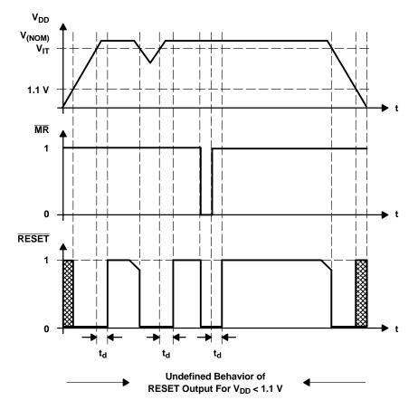
NOTE:  $\overline{\text{RESET}}$  should not be forced high during the power-up sequence (until  $V_{DD} > 1.1 \text{ V}$ ).
