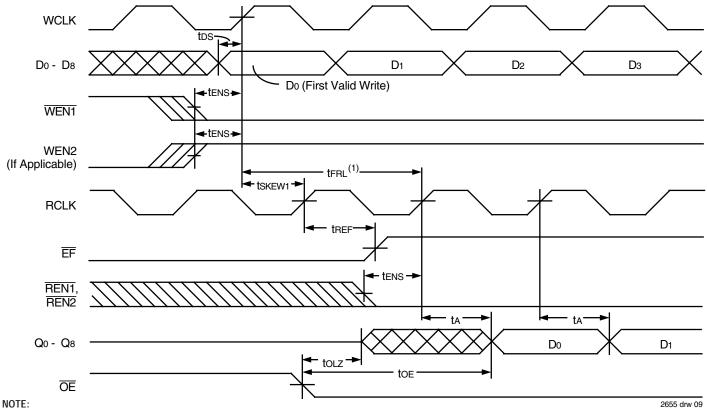
1. When tskew1  $\geq$  minimum specification, tfrl = tclk + tskew1 tskew1 < minimum specification, tfrl = 2tclk + tskew1 or tclk + tskew1. The Latency Timings apply only at the Empty Boundary ( $\overline{\text{EF}}$  = LOW).
