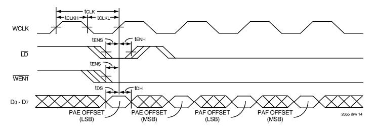
Figure 12. Write Offset Registers Timing
