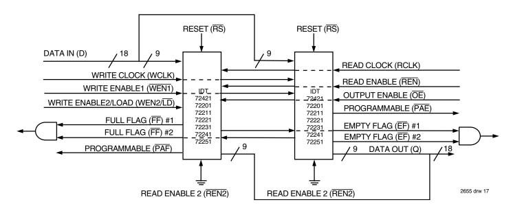
Figure 15. Block Diagram of 64 x 18, 256 x 18, 512 x 18, 1,024 x 18, 2,048 x 18, 4,096 x 18, 8,192 x 18
