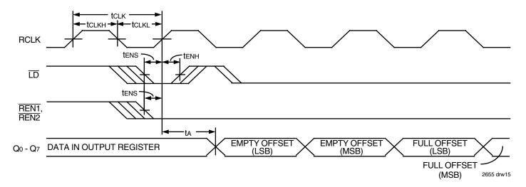
Figure 13. Read Offset Registers Timing
