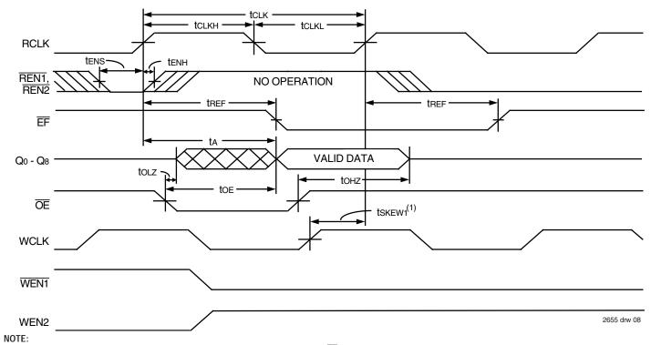
1. tskew1 is the minimum time between a rising WCLK edge and a rising RCLK edge for EF to change during the current clock cycle. If the time between the rising edge of RCLK and the rising edge of WCLK is less than tskew1, then EF may not change state until the next RCLK edge.
