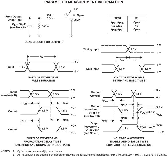
B. All input pulses are supplied by generators having the following characteristics: PRR ≤ 10 MHz, 2<sub>O</sub> = 50 Ω, t<sub>f</sub> ≤ 2.5 ns, t<sub>f</sub> ≤ 2.5 ns.
