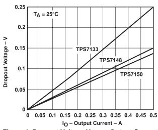
Figure 1. Dropout Voltage Versus Output Current
