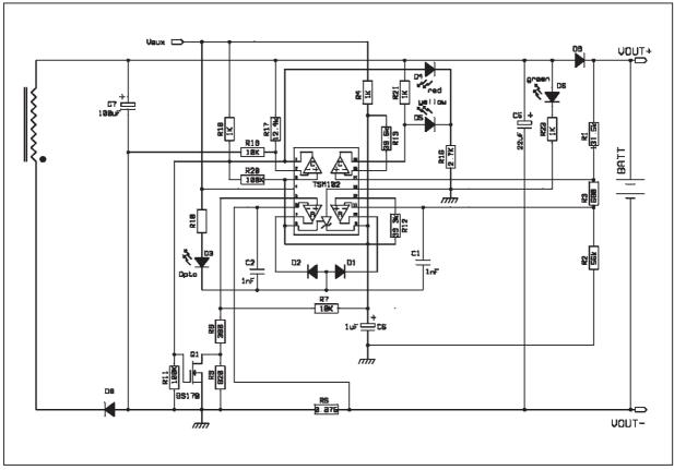
Figure 2: The Application Schematic - Battery Charger Secondary Side
