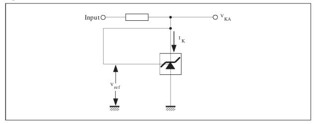
Figure 2: Test Circuit for  $V_{KA} > V_{ref}$
