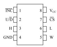
8-Pin DIP (300mil) 8-Pin SO (150mil) 8-Pin µSOP (118mil) 8-Pin Flip-Chip Package
