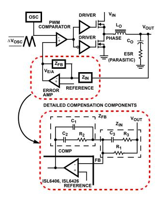
FIGURE 7. VOLTAGE-MODE BUCK CONVERTER COMPENSATION DESIGN
