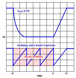
FIGURE 5. OVERCURRENT PROTECTION RESPONSE
