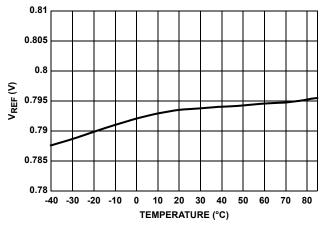
FIGURE 1. REFERENCE VOLTAGE vs TEMPERATURE
