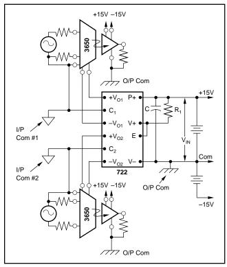
FIGURE 2. Two-Port Isolation with Two 3650s.
