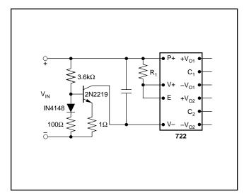
FIGURE 3. Short-Circuit Protection.
