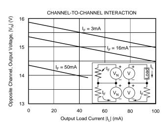
NOTES: (1) Using a 104mm x 19mm x 1.6mm aluminum strip mounted to the bottom of the case with heat sink compound. (2) Total output current is the sum of the currents for each individual output.
