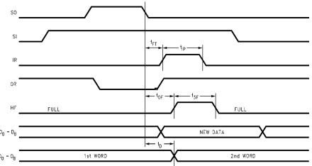
Note:  $\overline{\text{MR}}$  and FULL are HIGH;  $\overline{\text{OE}}$  is LOW.
