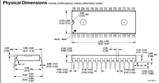
28-Lead Plastic Dual-In-Line Package (PDIP), JEDEC MS-010, 0.600" Wide Package Number N28B
