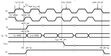
Note: SI and  $\overline{\text{OE}}$  are LOW;  $\overline{\text{MR}}$  is HIGH; D<sub>0</sub>–D<sub>8</sub> are immaterial.
