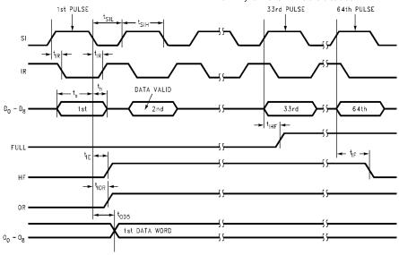
Note: SO and  $\overline{\text{OE}}$  are LOW;  $\overline{\text{MR}}$  is HIGH.
