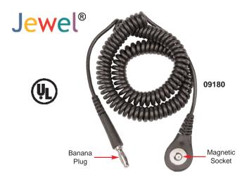
Jewel® MagSnap Coil Cords meet or exceed the requirements of ANSI/ESD S20.20 and ANSI/ESD S1.1 including section 5.4 Breakaway Force "With the ground cord connected to the cuff in a normal manner, a force of  $\geq$  .45 kg (1 lb) but  $\leq$  2.3 kg (5 lb) applied to the ground cord, in the normal disconnect direction, shall be required to separate the ground cord from the cuff."
