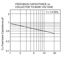
VcB-Collector to Base Voltage-V
