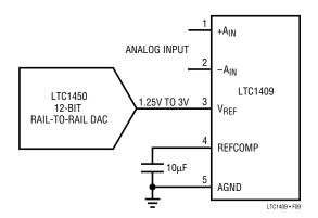
Figure 9. Driving V<sub>REF</sub> with a DAC
