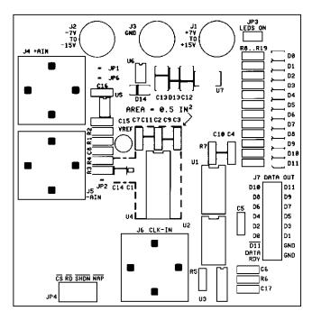
Figure 13b. Suggested Evaluation Circuit Board Component Side Silkscreen
