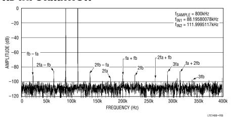
Figure 5. Intermodulation Distortion Plot
