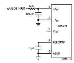
Figure 7a. RC Input Filter
