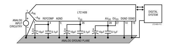
Figure 12. Power Supply Grounding Practice
