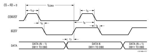
Figure 17. Mode 1b. CONVST Starts a Conversion. Data Outputs Always Enabled
