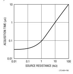
Figure 6. Acquisition Time vs Source Resistance
