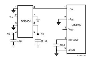
Figure 7b. 500kHz 5th Order Elliptic Lowpass Filter
