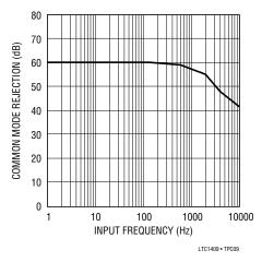
Figure 10a. CMRR vs Input Frequency
