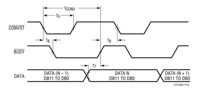
Figure 16. Mode 1a. CONVST Starts a Conversion. Data Outputs Always Enabled (CONVST = \\_\_\_\_\_\_\_\_)
