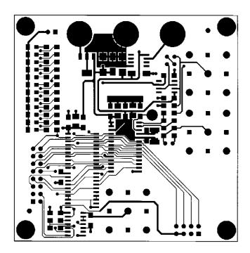
Figure 13c. Suggested Evaluation Circuit Board Component Side Layout
