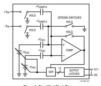
Figure 1. Simplified Block Diagram
