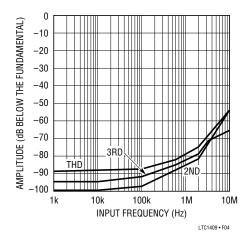
Figure 4. Distortion vs Input Frequency
