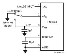
Figure 10b. Selectable 0V to 5V or ±2.5V Input Range
