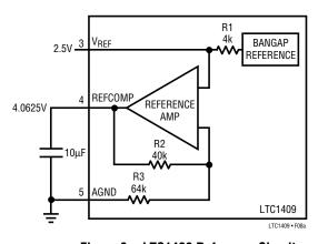
Figure 8a. LTC1409 Reference Circuit
