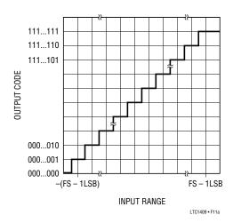
Figure 11a. LTC1409 Transfer Characteristics
