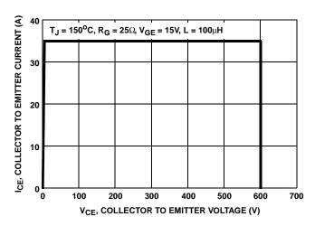
FIGURE 2. MINIMUM SWITCHING SAFE OPERATING AREA
