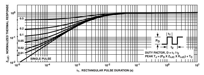
FIGURE 19. IGBT NORMALIZED TRANSIENT THERMAL RESPONSE, JUNCTION TO CASE
