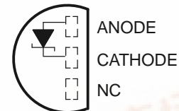
LP (TO-92/TO-226) PACKAGE (TOP VIEW)
