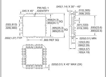
**84J**, 84-Lead, Plastic J-Leaded Chip Carrier (PLCC) Dimensions in Inches and (Millimeters)
