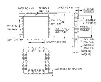
**68J**, 68-Lead, Plastic J-Leaded Chip Carrier (PLCC) Dimensions in Inches and (Millimeters)
