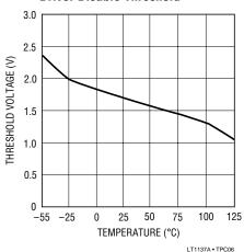
**ON/OFF** Thresholds 3.0 2.5 THRESHOLD VOLTAGE (V) 2.0 ON THRESHOLD 1.5 1.0 OFF THRESHOLD 0.5 0 -55 -25 0 25 50 75 100 125 TEMPERATURE (°C) LT1137A • TPC07
