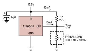
\*SELECT R1 TO DELIVER 80% OF TYPICAL LOAD CURRENT. LT1460 WILL THEN SOURCE AS NECESSARY TO MAINTAIN PROPER OUTPUT. DO NOT REMOVE LOAD AS OUTPUT WILL BE DRIVEN UNREGULATED HIGH. LINE REGULATION IS DEGRADED IN THIS APPLICATION
