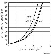
Output Voltage Temperature Drift
