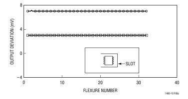
Figure 8a. Same Two LT1460S8-10s in Figure 7a, but With Slots
