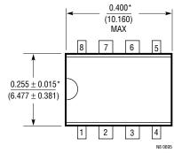
\*THESE DIMENSIONS DO NOT INCLUDE MOLD FLASH OR PROTRUSIONS. MOLD FLASH OR PROTRUSIONS SHALL NOT EXCEED 0.010 INCH (0.254mm)
