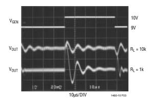
Figure 3.  $C_L = 0.01 \mu F$
