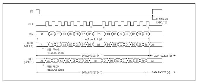
Figure 5. Serial-Interface Timing Diagram
