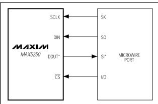
\*THE DOUT-SI CONNECTION IS NOT REQUIRED FOR WRITING TO THE MAX5250, BUT MAY BE USED FOR READBACK PURPOSES.
