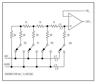
Figure 1. Simplified DAC Circuit Diagram
