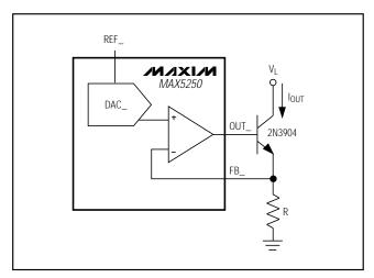
Figure 13. Digitally Programmable Current Source
