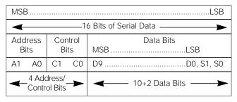
Figure 4. Serial-Data Format
