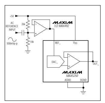
Figure 12. AC Reference Input Circuit
