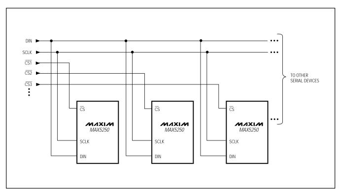
Figure 8. Multiple MAX5250s Sharing a Common DIN Line
