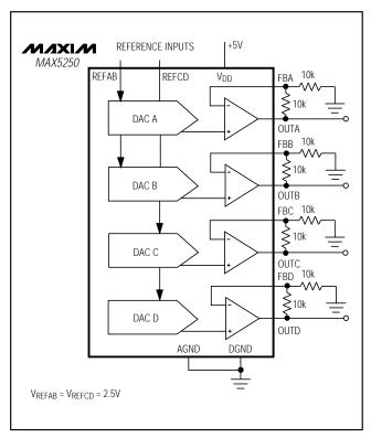
Figure 10. Unipolar Rail-to-Rail Output Circuit
