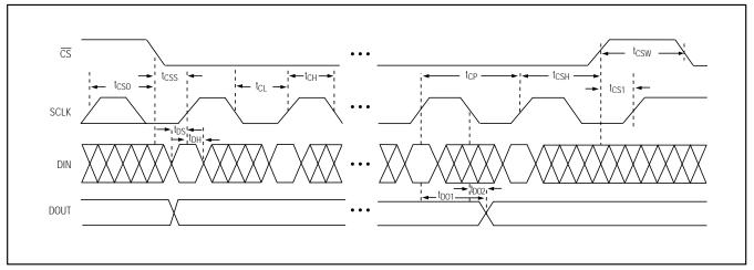
Figure 6. Detailed Serial-Interface Timing Diagram
