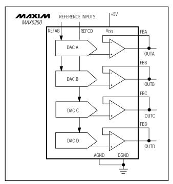
Figure 9. Unipolar Output Circuit
