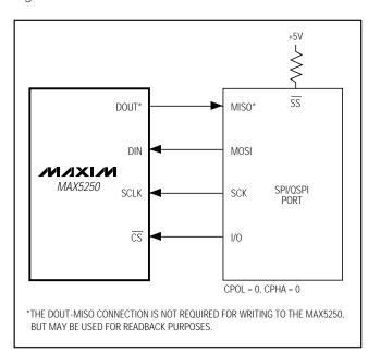
Figure 3. Connections for SPI/QSPI
