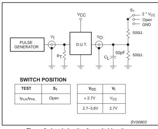
Figure 2. Load circuitry for switching times.
