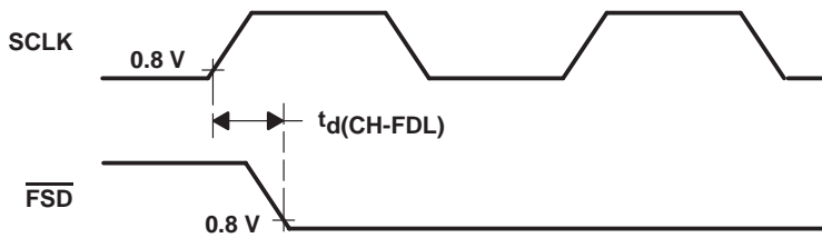
Figure 5–3. Master/Slave SCLK to \overline{\text{FSD}} Timing
